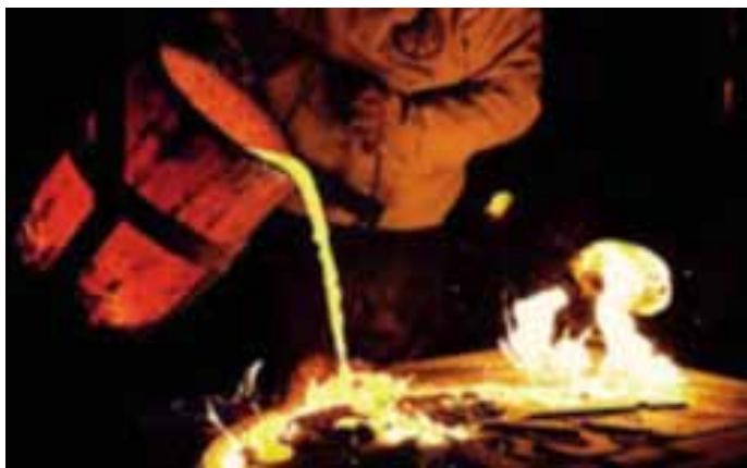
Casting - bronze is melted to a temperature 1100°C and poured into the mould cavity
