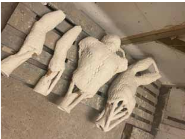
Waxes encased in ceramic shells, Fig C
